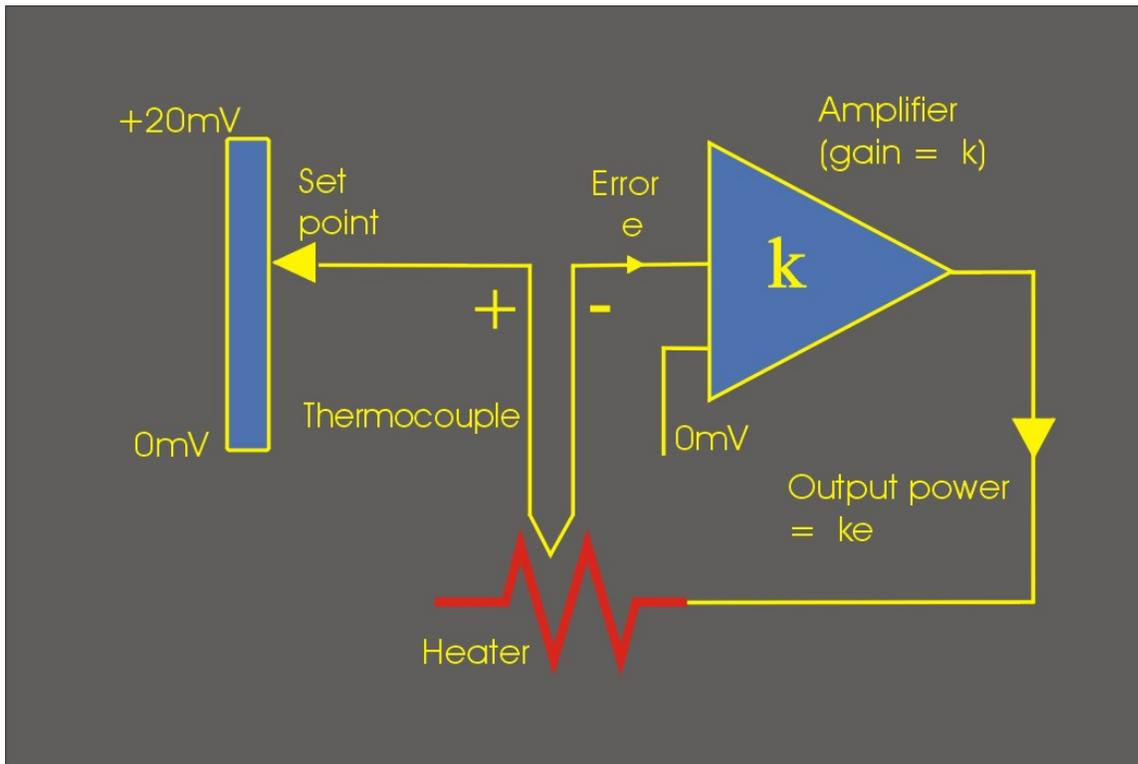
Fig 3. Simple controller circuit with thermocouple and load
