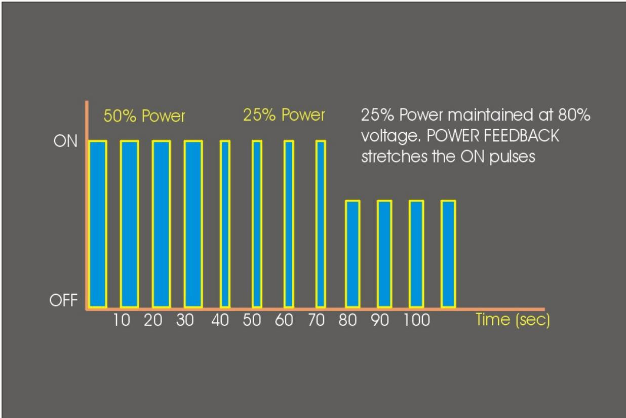
Fig 4. Modulation of power by pulse width variation
