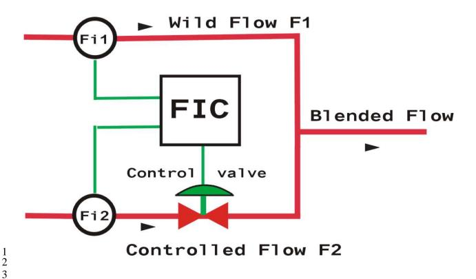
**Mixing and blending two liquids.** Fig 1 shows two streams, **wild flow** F1 and **controlled flow** F2 that converge to make the blended flow (the wild flow may be controlled somewhere upstream and is not necessarily wild). The controller's job is to drive F2 to a value that assumes the chosen preset ratio to F1.
