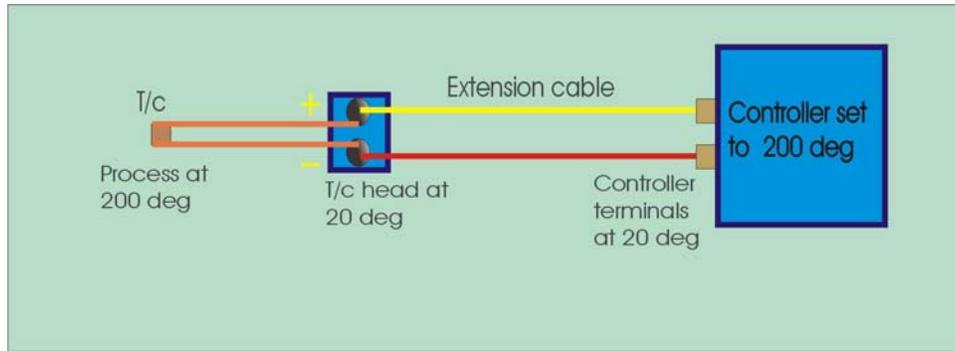
**Fig 1. Thermocouple wiring**
