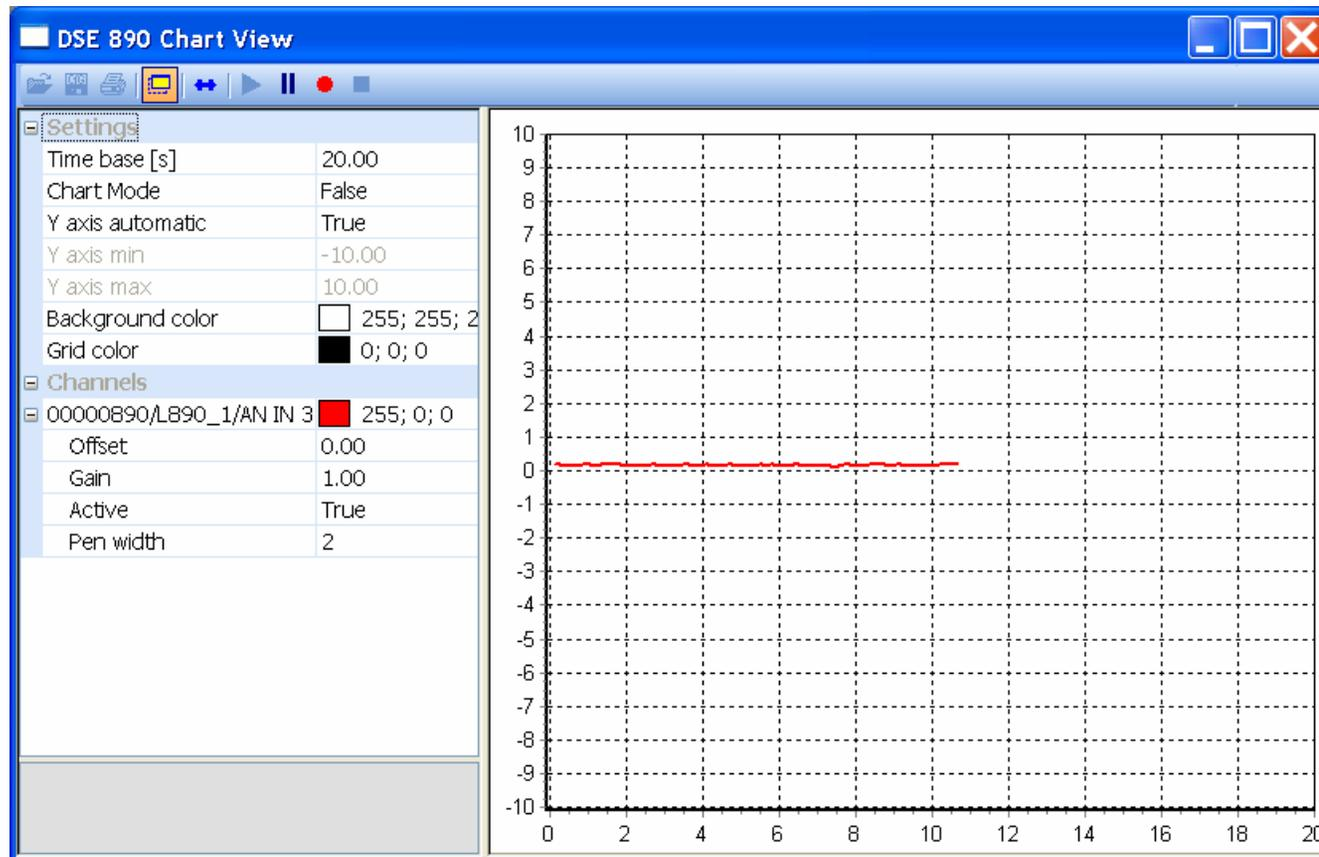
Here is a typical chart. It shows one parameter, analog input 3 "AN IN 3".
