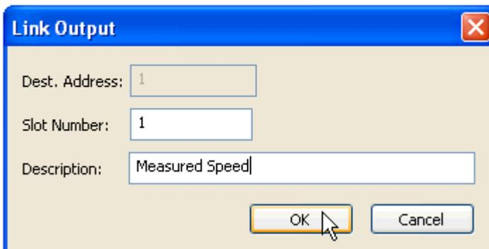
Similarly, a slot Output will ask you for the destination slot number (for standalone configurations, the Dest. address is fixed to be the same as the configuration's address). Again, the Description field is optional.
