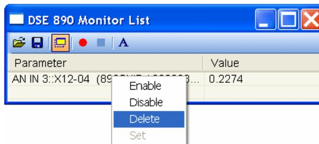
You can easily remove a parameter from the Monitor List by a right click and selecting "Delete".
