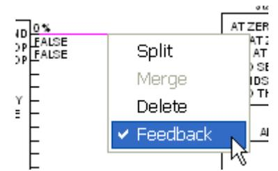
cursor to an 'x' to give visual feedback that the cursor is over an output and that the user can start drawing a connection. While holding the left mouse button down, drag the mouse cursor to start drawing the link. The link being drawn will be displayed in red, by default, and when you move the cursor over a valid input it will turn green, by default, to indicate that you have a valid link selected. Let up on the mouse button to make the connection.
