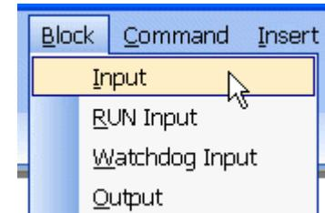
address to the configuration in which they reside. Slot inputs and outputs are selected from the top of the Block menu. There are three types of inputs ('Input', 'Run Input' and 'Watchdog Input'). All three of these inputs will request you to specify a 'slot' number when inserting them in the configuration. This slot number is what is used by the external device to identify this input. The Source and Description fields are optional.
