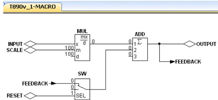
Let's say you wanted the second input to the macro to be RESET and the third to be SCALE. Click on SCALE with the right mouse button and select Move 'SCALE' Down
