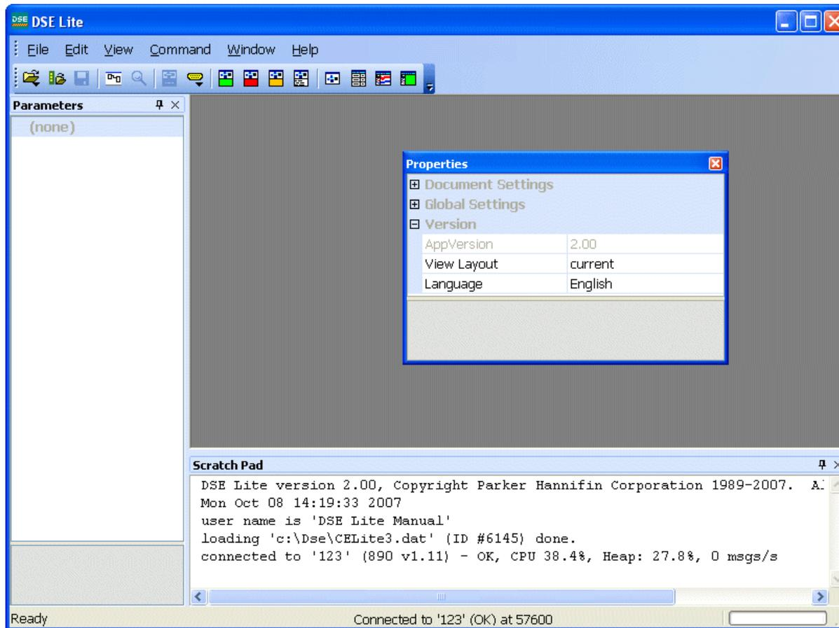
One is the ‘Parameters’ windows which is ‘docked’ to the left side of the main window. Another is the ‘Scratch Pad’ which is ‘docked’ to the bottom of the main window. Finally, the ‘Properties’ window is ‘floating’ near the center of the main window. We’ll talk about what each of these and other docking windows do later, but for now we’re going to discuss how to view, hide, move, dock and undock these windows.
