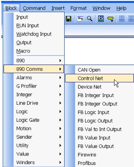
As you can see, there are many supported field bus (there may be others not displayed here). The function blocks that begin with 'FB' are input and output blocks shared by all of the various field buses. They are used vary similar to the *Link* inputs and outputs described above with the exception that there is no slot number (this is assigned internally when you configure the field bus, see example for Control Net), you need to pick the correct block depending on the data type of
