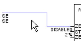
Selecting Feedback flags the link as a feedback (for drives that have feedback links). Feedback links are shown as a different color, light blue by default. Most drives update all pre-defined function blocks at a periodic rate or scan. Feedback links are processed at the end of that scan
