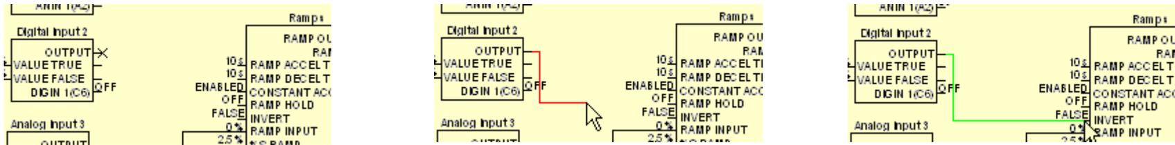
will change color to indicate that it is selected. Drag the mouse while holding down the mouse button to change the shape of the link.
